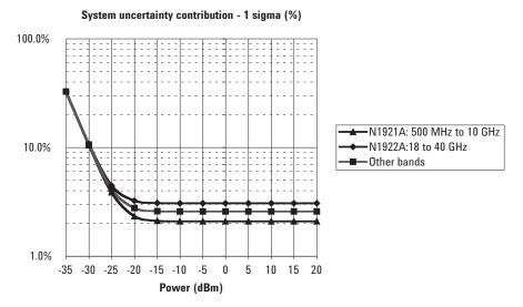
Note: The above graph is valid for conditions of free-run operation, with a signal within the video bandwidth setting on the system. Humidity < 70%.
