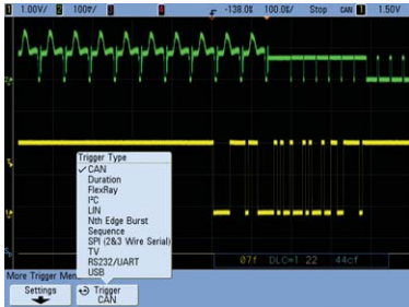
Trigger on and decode CAN serial packets.
