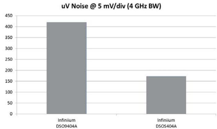
Superior signal integrity allows for more accurate measurements such as rise time values. Extremely low intrinsic jitter (100 fs) ensures the lowest possible contribution to jitter measurements from the scope itself so you're using your jitter budget on your design.
