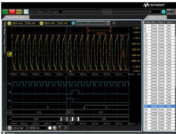
Use the digital channels to evaluate control signal relationships and data buses up to 16 bits wide. Use symbols to quickly interpret waveforms.
