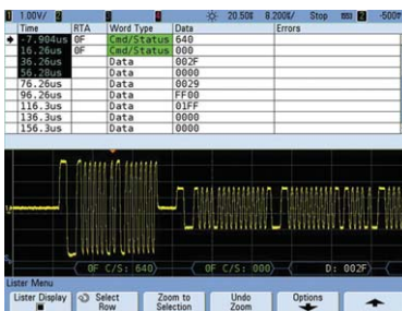
Figure 12. Time-correlated display of the MIL-STD 1553 physical layer signal with protocol decoding.
