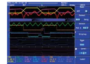
8-channel analog and 16-bit logic display
