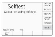
Selecting 'PRINTER' transfers to the 'Printer test.' screen. This invites a user to use a printer to test the interface (e.g. by switching the printer off-line, or removing the paper), and reports on the status of the printer:
