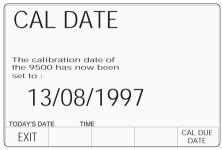
The alpha-numeric keypad is locked out. If updating the date-stamp is all that is required, without altering the due date, press the **EXIT** screen key to return to the **Mode Selection** screen.
