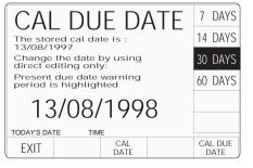
This screen also displays a stored CAL DATE reminder for calculating the cal due date.
