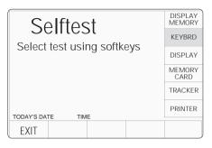
Selecting 'KEYBRD' transfers to the 'Keyboard test.' screen. This invites a user to press the front panel key to be tested, and reports on the screen the details of the last key to be pressed:
