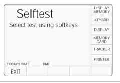
The required check can be selected from the list on the right of the screen, using the corresponding screen key.
