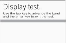
The screen text will shift automatically so as not to obscure the band as it jumps back to the top of the screen. If there are elements of the screen which do not show light in the light background or dark in the dark band as it is advanced down the screen, then this implies a failure. Rectification will require access to the internal circuitry, so no further user action is recommended, except to report the result to your Wavetek Service Center.
