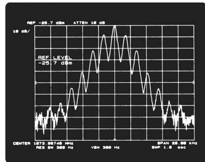
3. Third, press [REFERENCE LEVEL.] and raise the signal under test to the top graticule line of the CRT.
