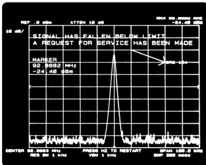
Use the command flow functions to monitor a desired signal level. If the signal goes below the specified level, alert a computer by setting an GP-IB service request. This will interrupt current computer operations and allow appropriate action to be taken.
