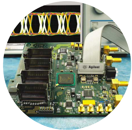
Figure 3. Agilent's soft touch probes combine high-density, low loading and differential capability into a reliable, space-saving package.
