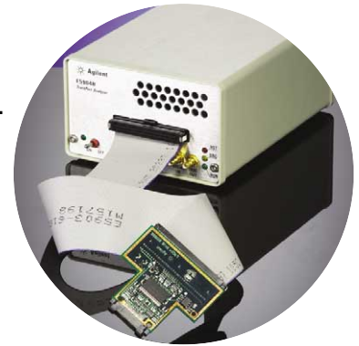
Figure 15. The Agilent E5904B trace port analyzer.
