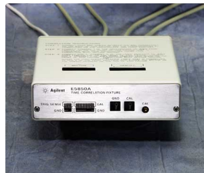
Figure 5.26. E5850A time correlation fixture.
