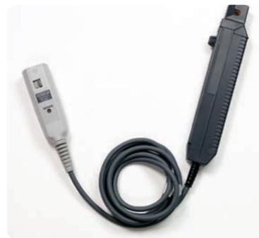
N2893A 100-MHz current probe with AutoProbe interface
