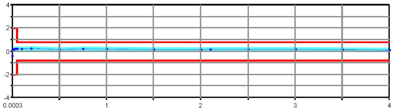
Output power accuracy in dB versus frequency in GHz of the R&S<sup>®</sup>ZVB4.
