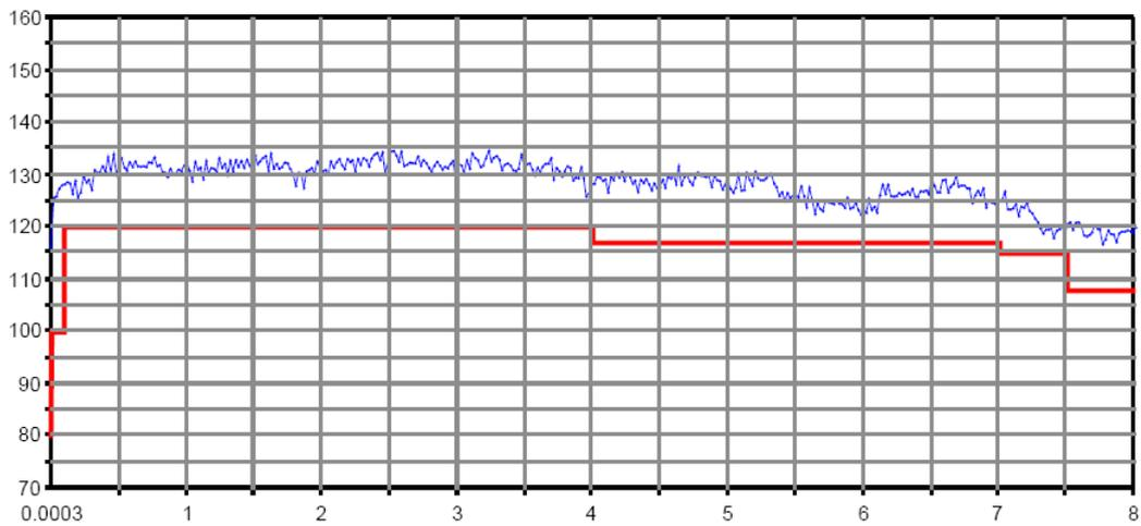
Dynamic range in dB versus frequency in GHz of the R&S<sup>®</sup>ZVB8.
