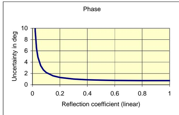
*Typical accuracy of reflection magnitude and reflection phase measurements of the R&S®ZVB4 in the frequency range from 300 kHz to 4 GHz, of the R&S®ZVB8 in the frequency range from 300 kHz to 8 GHz, of the R&S®ZVB14 in the frequency range from 50 MHz to 14 GHz, and of the R&S®ZVB20 in the frequency range from 50 MHz to 20 GHz.*
