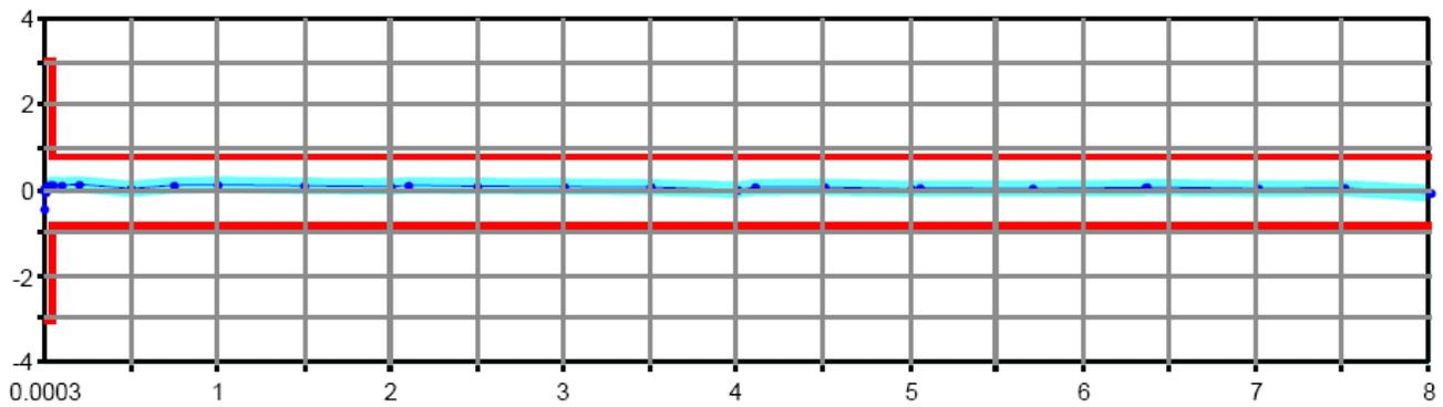
Output power accuracy in dB versus frequency in GHz of the R&S<sup>®</sup>ZVB8.
