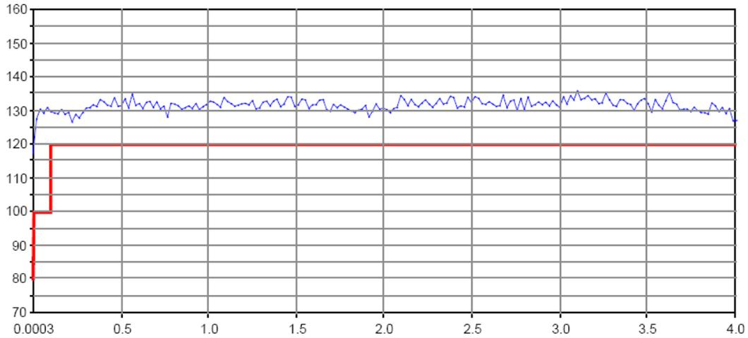
Dynamic range in dB versus frequency in GHz of the R&S<sup>®</sup>ZVB4.
