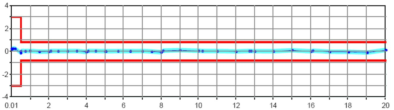
Output power accuracy in dB versus frequency in GHz of the R&S<sup>®</sup>ZVB14 (up to 14 GHz) and the R&S<sup>®</sup>ZVB20.
