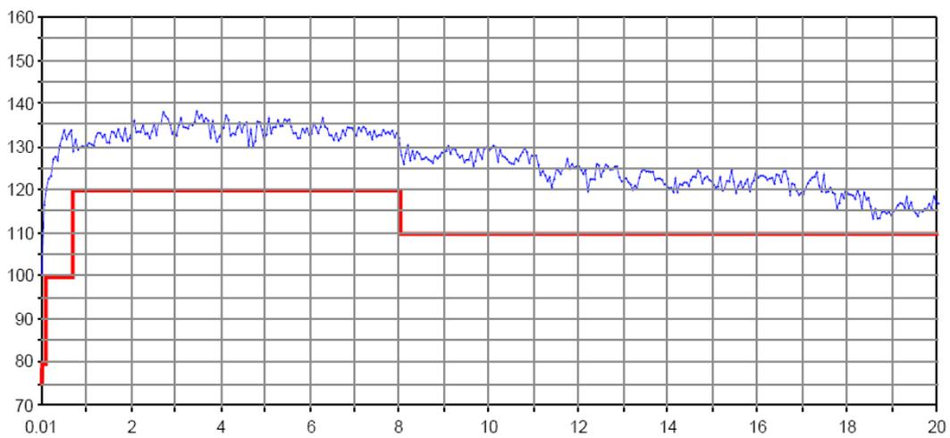
Dynamic range in dB versus frequency in GHz of the R&S<sup>®</sup>ZVB14 (up to 14 GHz) and the R&S<sup>®</sup>ZVB20.
