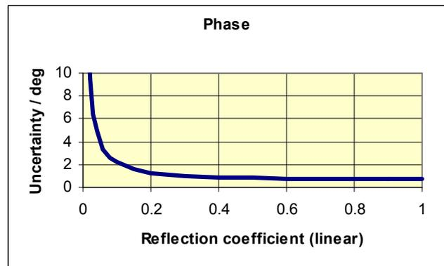
*Typical accuracy of reflection magnitude and reflection phase measurements of the R&S®ZVA8 in the frequency range 1 MHz to 8 GHz, of the R&S®ZVA24 in the frequency range 50 MHz to 24 GHz, of the R&S®ZVA40 in the frequency range 50 MHz to 40 GHz, of the R&S®ZVA50 in the frequency range 50 MHz to 50 GHz and of the R&S®ZVA67 in the frequency range 50 MHz to 67 GHz.*
