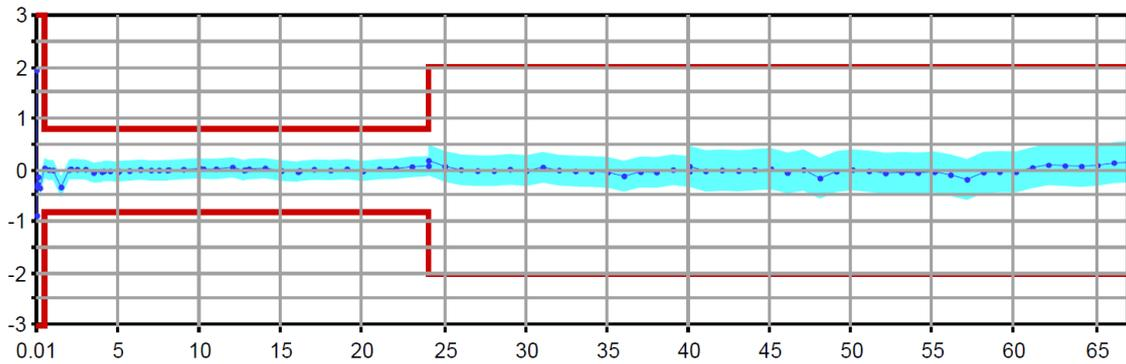
Output power accuracy in dB versus frequency in GHz of the R&S®ZVA67.
