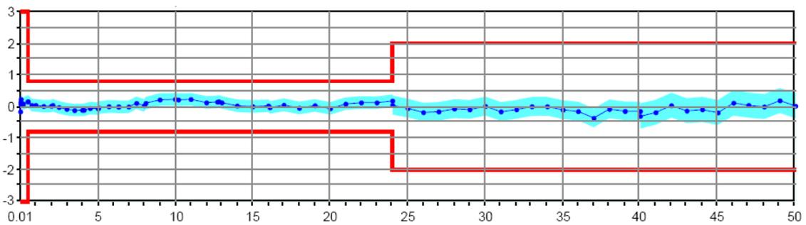
Output power accuracy in dB versus frequency in GHz of the R&S<sup>®</sup>ZVA50
