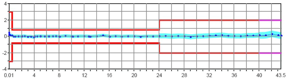
Output power accuracy in dB versus frequency in GHz of the R&S<sup>®</sup>ZVA40
