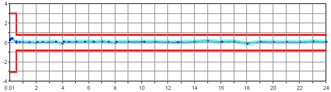
Output power accuracy in dB versus frequency in GHz of the R&S<sup>®</sup>ZVA24
