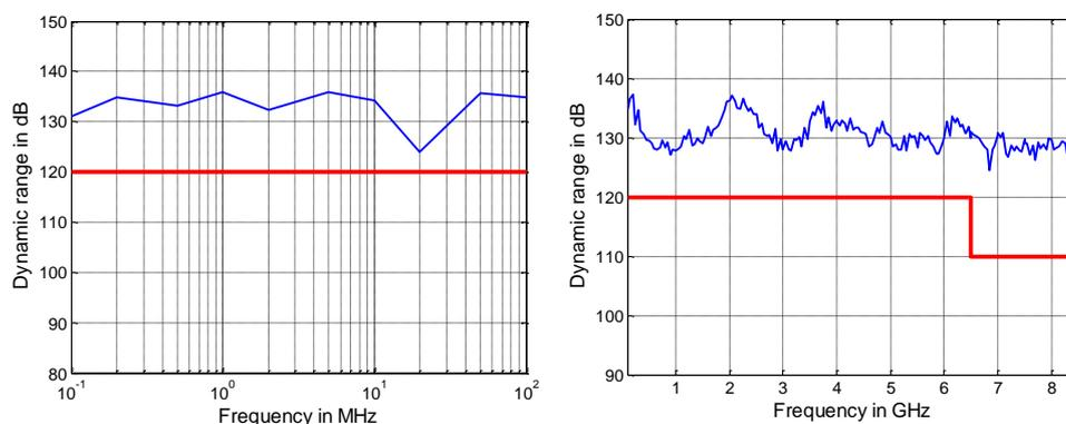
Dynamic range in dB versus frequency for the R&S<sup>®</sup>ZND base unit
