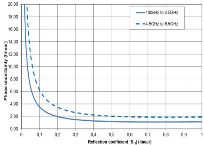
Typical accuracy of reflection magnitude and reflection phase measurements for the R&S®ZND;
