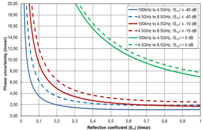
Typical accuracy of reflection magnitude and reflection phase measurements for the R&S®ZND;
