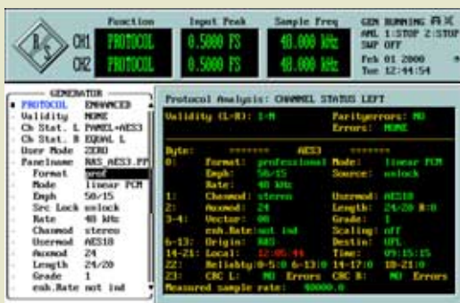
Fig. 12: The R&S UPL generates and analyzes additional data in digital data streams in line with all common standards. The data is represented in binary form, as hexadecimal numbers, or as ASCII characters, or it is evaluated in consumer or professional format.
