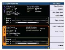
Figure 1: Configure your digital generator DSI settings, including the output format of your choice. Choose amongst four formats: I<sup>2</sup>S, Left Justified, Right Justified and DSP
