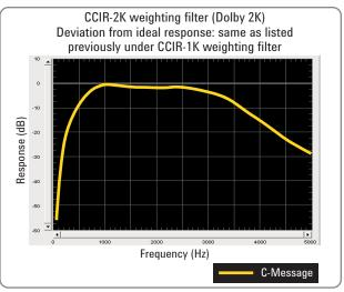
Figure 15. CCIR-2K weighting filter
