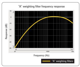
Figure 14. "A" weighting filter frequency response
