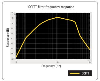
Figure 17. CCITT filter frequency response
