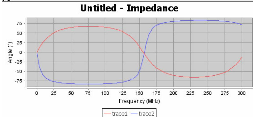
The new trace will be plotted in the same chart as the original and a legend will indicate the colour of each trace. Individual traces may be displayed or hidden on the chart area by checking or un-checking the **Display on Chart** checkbox in the control panel trace group.
