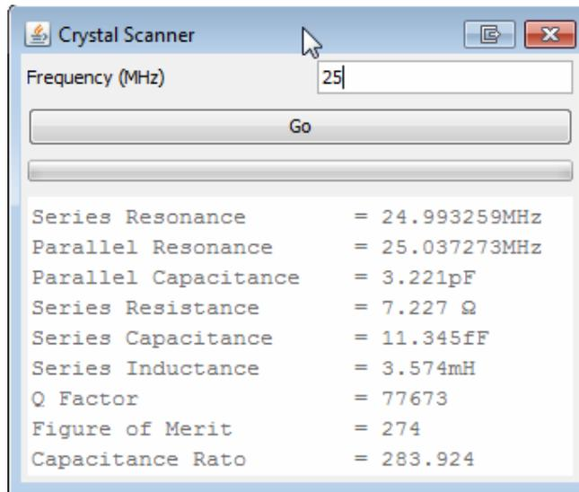
All parameters are measured or calculated and displayed on the screen. These values are automatically copied to the clipboard for pasting into other application.
