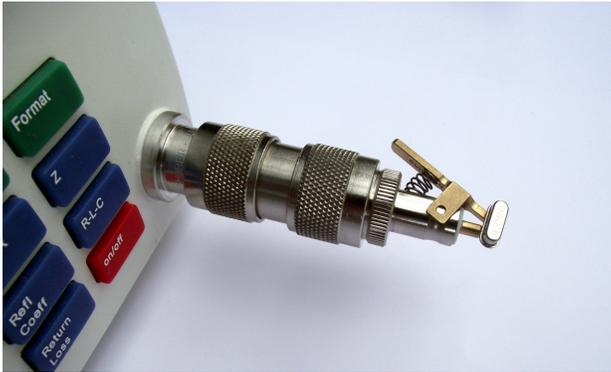
Once the measurement fixture is calibrated out, the crystal scan function can be used to measure the crystal parameters.
