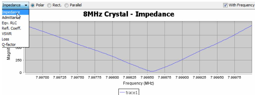
In the example above, **Impedance** is chosen from the drop list and the **Polar** radio button is selected. So this is a plot of Polar Impedance vs Frequency.
