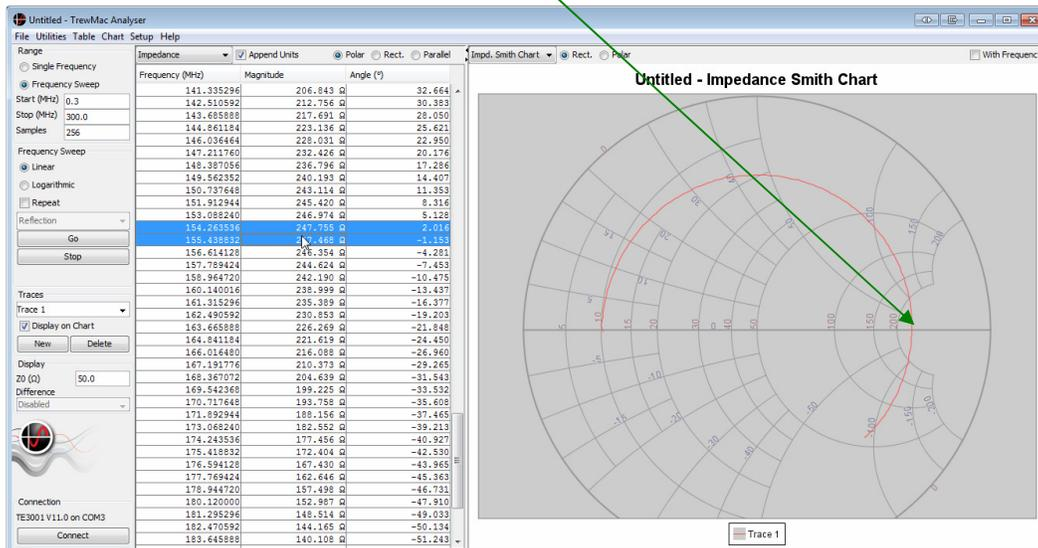
The Velocity Factor  $VF = \frac{mf}{4C}$  where m is the length in meters, f is the zero crossing frequency (quarter wave frequency) and C is the speed of light in a vacuum.
