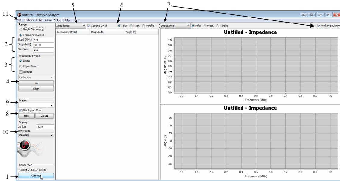
If an analyser is found, the type and port number will be displayed in the connection area at the bottom of the control panel (1). If no analyser is detected, check the connection to the PC and press the **Connect** button in the connection area (1). For issues with the USB connection, see the Installation section of this manual.
