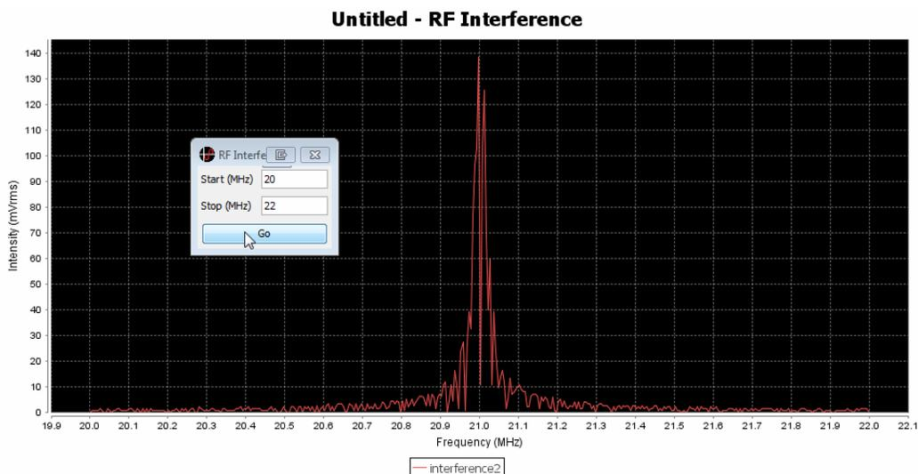
The image above shows an interference scan from 20-22MHz. A signal generator generates -10dBm sinusoidal interference at 21MHz.
