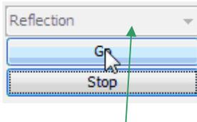
The Sweep **Mode** drop box (lowest position in the sweep group) is for 2 port operations and is locked to Reflection for single port usage. When using the TE3002 use this drop box to select between S11 reflection mode and S21 transmission mode.
