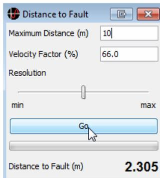
The unit will conduct a sweep with the required number of points, compute the inverse Fourier transform, and generate an Impulse data trace. The Distance to Fault is determined as the location of the highest peak in the new impulse trace and is displayed in the dialogue box.
