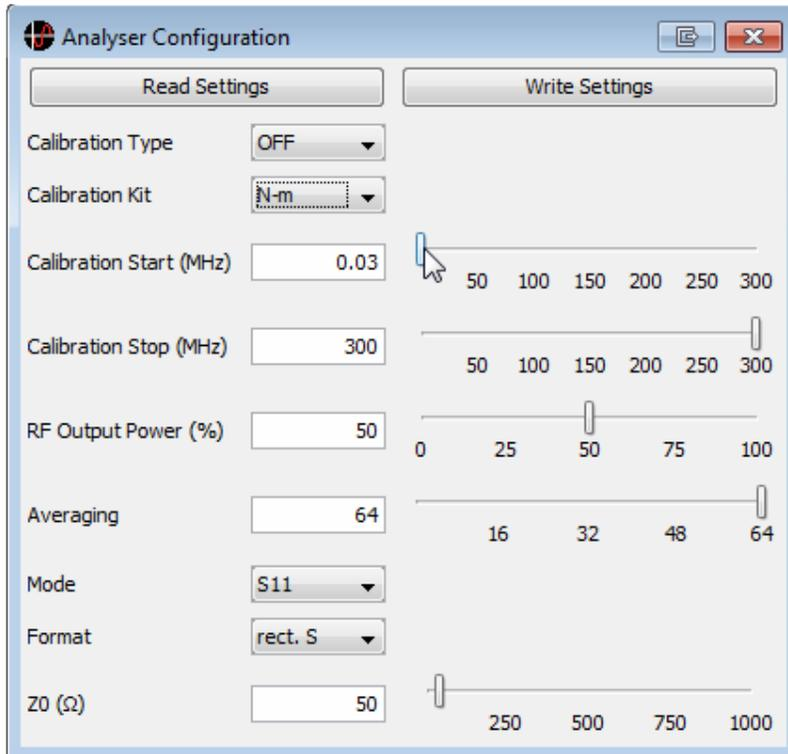
The analyser configuration window provides read/write access to the analyser's system parameters. All of these parameters are available on the analyser itself by pressing the **System Zo** or **Cal** key.
