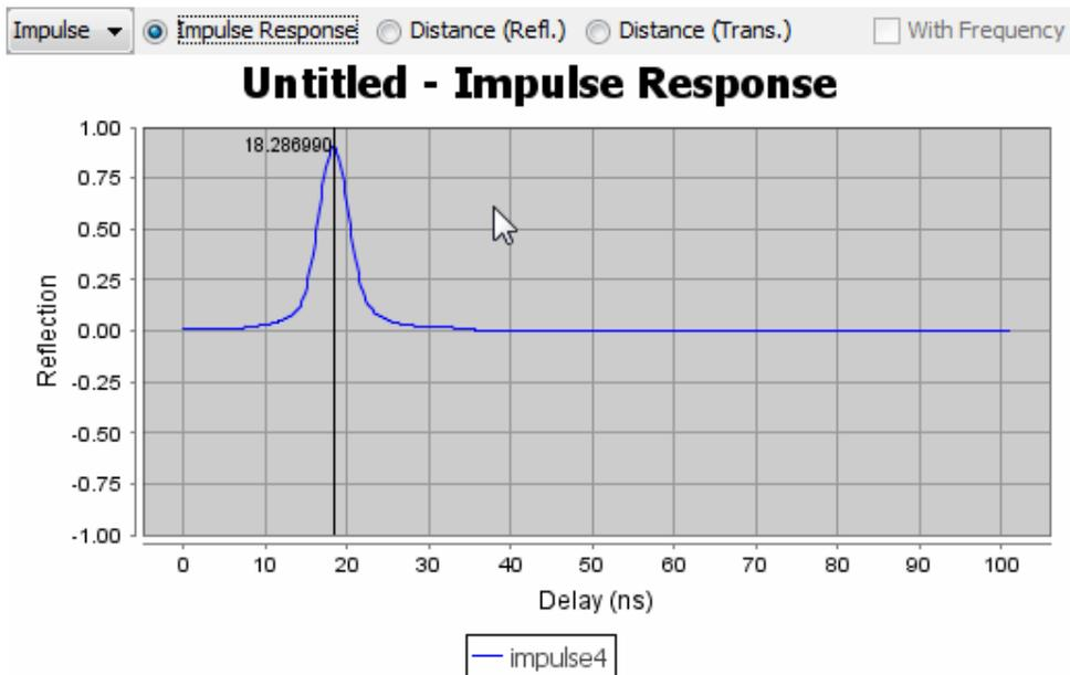
Any deviation from the normal characteristic impedance of the transmission line will generate a reflection. For example, a pinch in a length of 50 Ohm coaxial line may reduce the impedance at the pinch. This in turn will cause a negative going reflection (because it's less than  $Z_0$ ) at this point. A severed coaxial line will appear as an Open termination, resulting in a positive going reflection.
