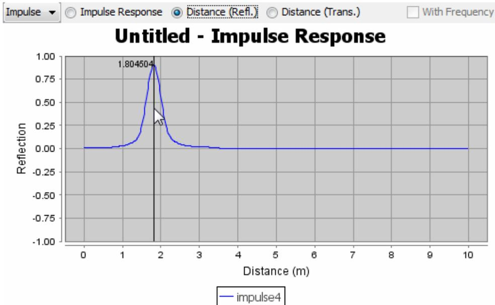
When the **Impulse Response** radio button is checked, the X axis is should be read as the time taken for the impulse to travel down the line and back again.
