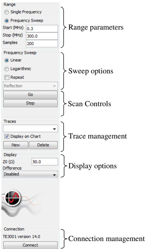
The control panel is divided into several functional sections, each indicated by a bracket on the right side:
