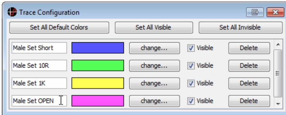
This window provides control over how the traces in the charts are plotted. The visibility, colour, and name of each trace may be set individually. Alternately the **Set All Visible/Invisible** buttons provides group control. Traces may be deleted but may not be restored after deletion.
