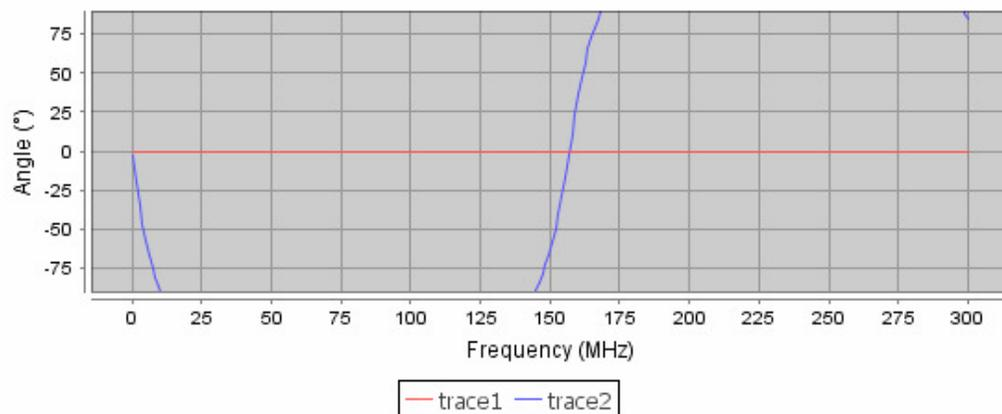
Of course, if trace1 is selected as the reference for the difference function, the plot for trace1 will appear as a flat zero. It could be hidden by un-checking the **Display on Chart** checkbox in the Trace group of the control panel.
