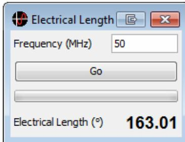
The utility will scan the transmission line and return the total electrical length.
