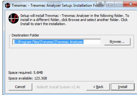
During normal installation, several windows may open and close as the serial port and USB drivers are installed on your computer.
