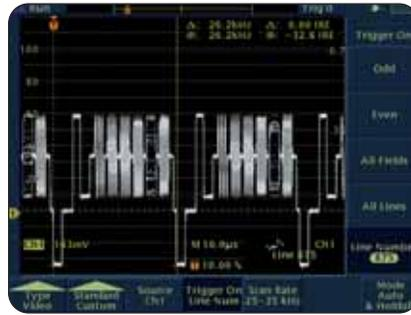
▶ Custom video trigger allows the TDS3000B to trigger on standards such as RS343 (26.2 kHz scan rate).
