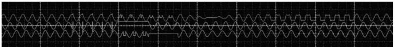
As shown by this photo, the SmartWave can create time coincident spikes on 3 phases, fractional or multi-cycle dropouts, sags and surges, waveforms distortion, DC and noise.
