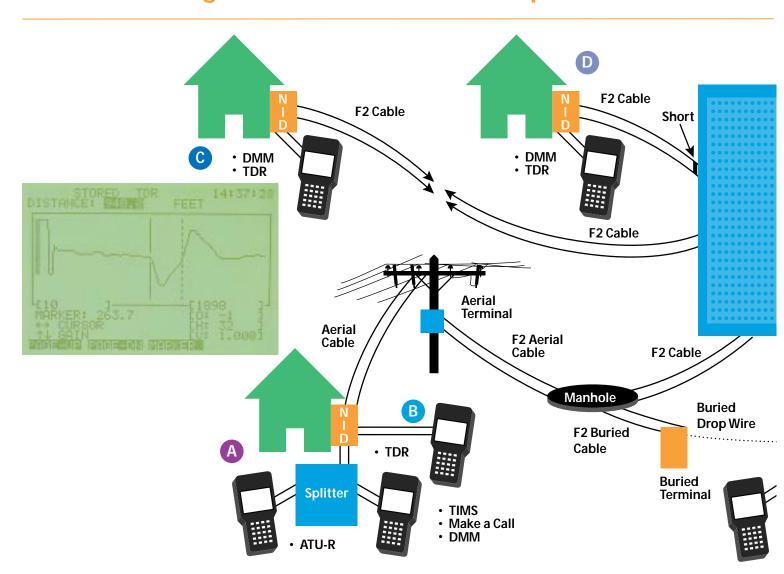
E This technician wanted to determine the loop length from the customer premises. So he called up the CO to place a hard metallic short on the line and used the loop resistance measurement to automatically calculate loop length. It was within specifications.
