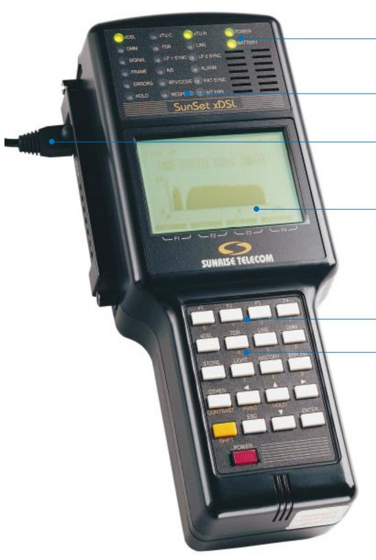
These indicators show battery charging from AC charging and give an early warning of battery failure.
