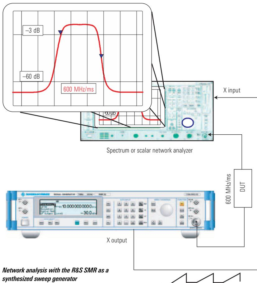
**Network analysis with the R&S SMR as a synthesized sweep generator**
