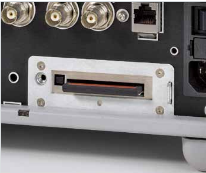
CompactFlash™ card ejector on instrument rear panel.
