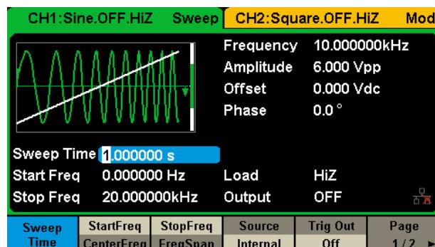
SDG2000X supports two Sweep modes, "Linear" and "Log". Two Sweep directions, "Up" and "Down" and three Sweep sources, "Internal", "External" and "Manual".
