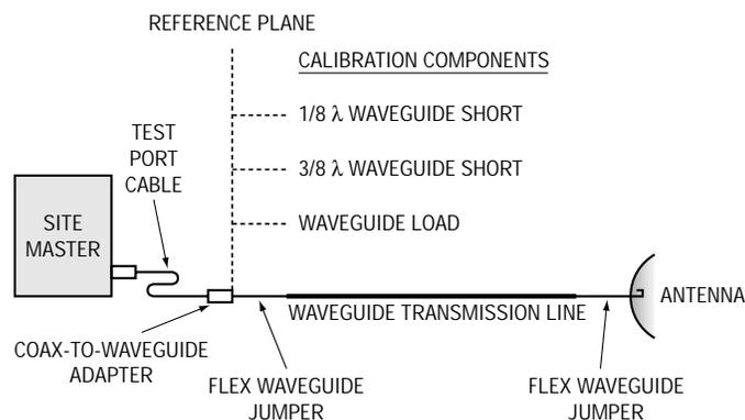
*Vector Correction Avoids Bulky Waveguide Coupler*
