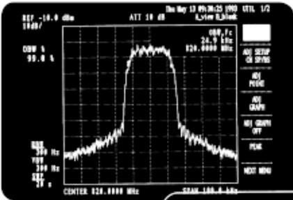
OBW (occupied bandwidth) display PDC 800 MHz band
