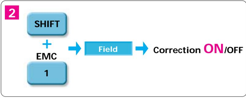
Set Correction to ON. The corrected data is reflected on the screen data.
