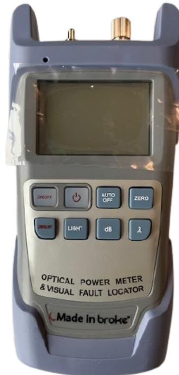
**LE MIB OPM + VFL PERMET D'IDENTIFIER DES FIBRES, DE MESURER L'ATÉNUATION OPTIQUE, DE VÉRIFIER LA CONTINUITÉ ET D'ÉVALUER LA QUALITÉ DE TRANSMISSION SUR LES FIBRES OPTIQUES MONOMODES ET MULTIMODES DANS L'INFRASTRUCTURE FTTH/ LAN/ WAN/ CATV .**
