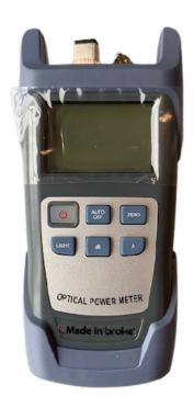
LE MIB OPM PERMET D'IDENTIFIER DES FIBRES, DE MESURER L'ATÉNUATION OPTIQUE, DE VÉRIFIER LA CONTINUITÉ ET D'ÉVALUER LA QUALITÉ DE TRANSMMITION SUR LES FIBRES OPTIQUES MONOMODES ET MULTIMODES DANS L'INFRASTRUCTURE FTTH/LAN/WAN/CATV.
