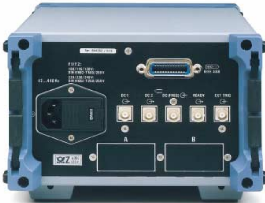
Rear panel view of NRVD
