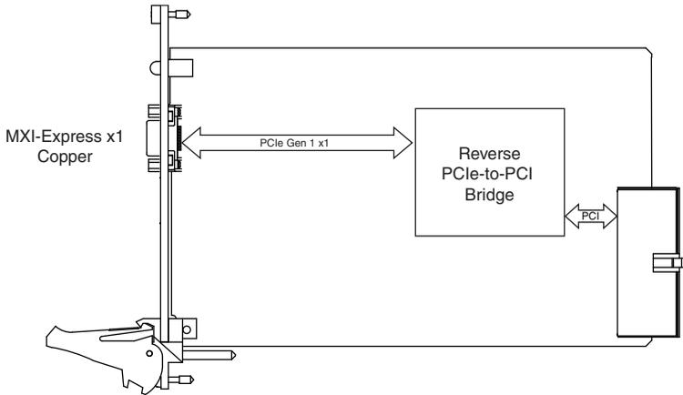
**Figure 1-7. NI PXI-8367 (199991x-04L) Block Diagram**
