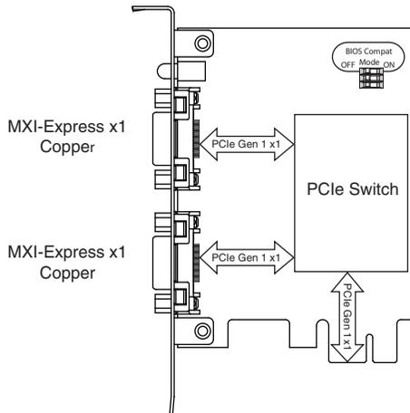
**Figure 1-5.** NI PXI-8360 (191373x-01) Block Diagram
