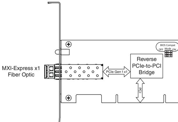
**Figure 1-3.** NI PCIe-8361 (199042x-01L) Block Diagram
