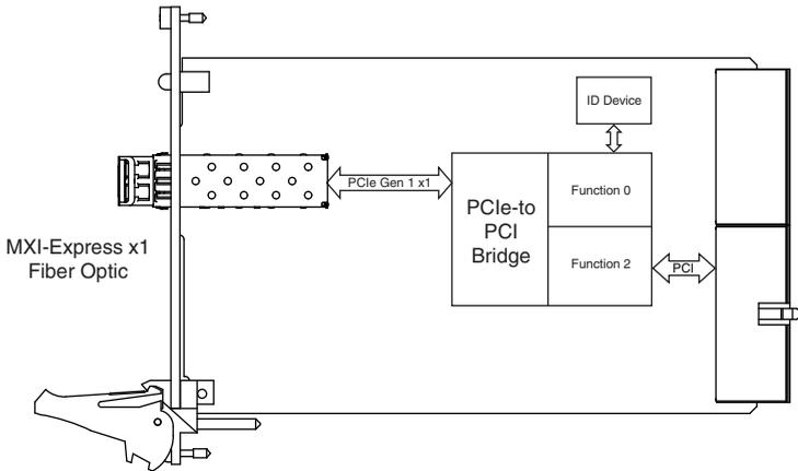
**Figure 1-9.** NI PXIe-8360 (194402x-01L) Block Diagram
