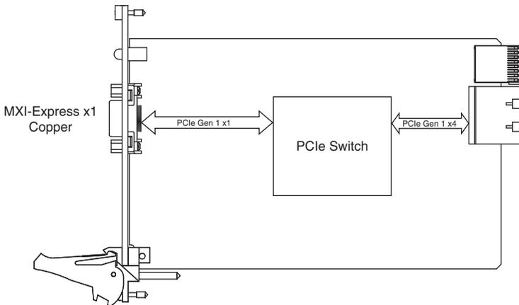
**Figure 1-11.** NI ExpressCard-8360 (198266x-01L) Block Diagram
