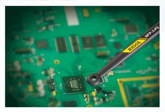
NFP-3-P4, a near-field probe which resolution is 2 mm. It can detect the vertically emitted electromagnetic field. It is applicable for the detection of magnetic field where current loop exists. For example, electromagnetic field testing for PCB wiring, magnetic field testing for IC pins area etc
