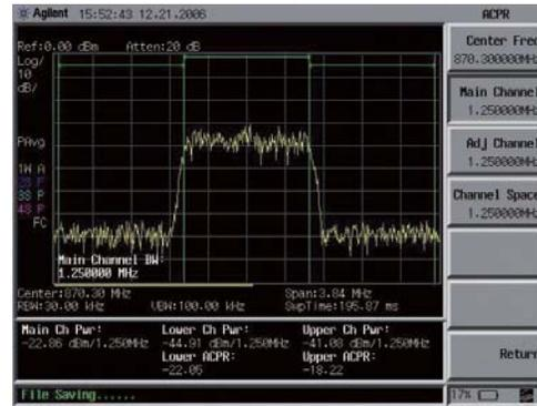
Center frequency, main channel bandwidth, adjacent channel bandwidth, and channel space can be set on the panel.
