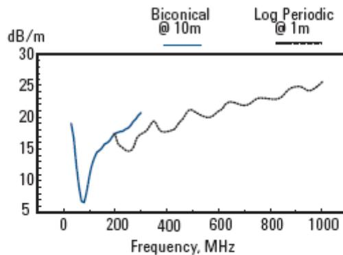
Linear units:  $AF = \text{Antenna factor (1/m)}$        $AF = \frac{E_{in}}{V_{out}}$
