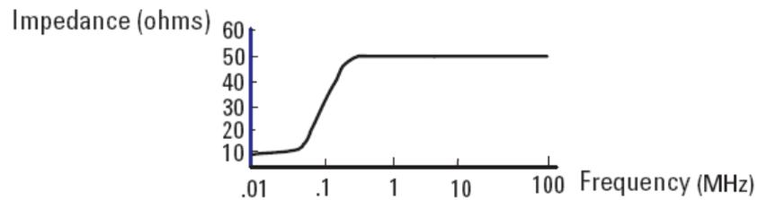
The 1 μF in combination with the 50 μH inductor is the filter that isolates the mains from the EUT. The 50 μH inductor isolates the noise generated by the EUT from the mains. The 0.1 μF couples the noise generated by the EUT to the X-Series signal analyzer or receiver. At frequencies above 150 kHz, the EUT signals are presented with a 50Ω impedance.
