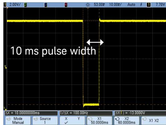
Figure 4. Voltage interrupt pulse generated by N7951A
