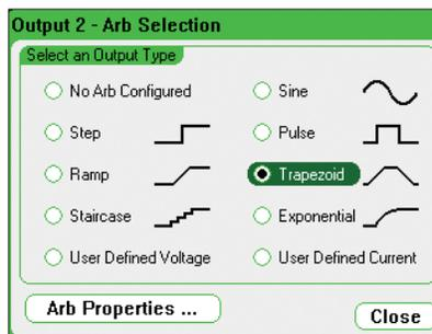
**Figure 8.** The Arb Selection menu is used to select which pre-programmed waveform will be applied to the output of the DC Power Module. Each of the four outputs can have a different waveform applied.
