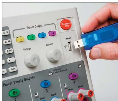
Figure 12. The N6705A's front panel USB port
