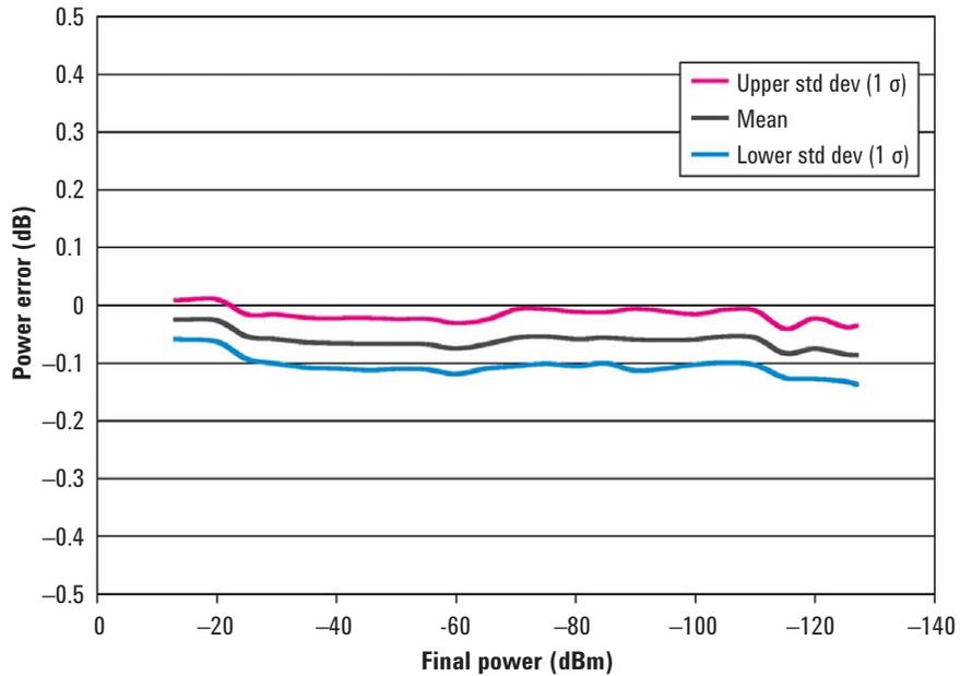
Relative level accuracy measures the accuracy of a step change from any power level to any other power level. This is useful for large changes (i.e. 5 dB steps).
