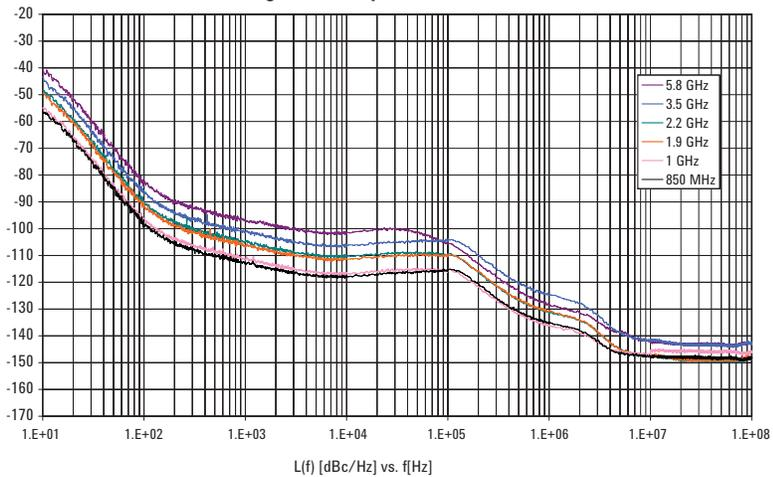
Single sideband phase noise optimized signal-to-noise floor mode<sup>1</sup>
