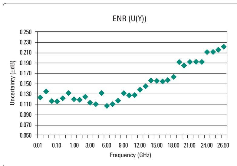
Figure 2. Characteristic ENR plot versus cardinal frequency points.
