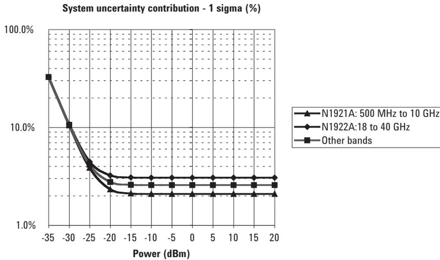
Note: The above graph is valid for conditions of free-run operation, with a signal within the video bandwidth setting on the system. Humidity < 70 %.
