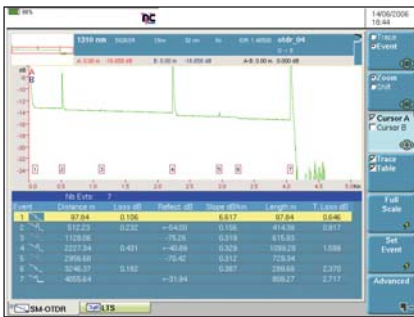
Trace and table displayed simultaneously
