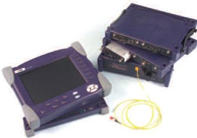
MTS-8000 field-scalable optical test platform
