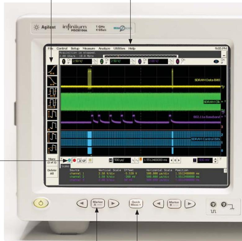
● **MegaZoom** technology enables you to quickly pan and zoom through the deepest waveforms for detailed analysis.
