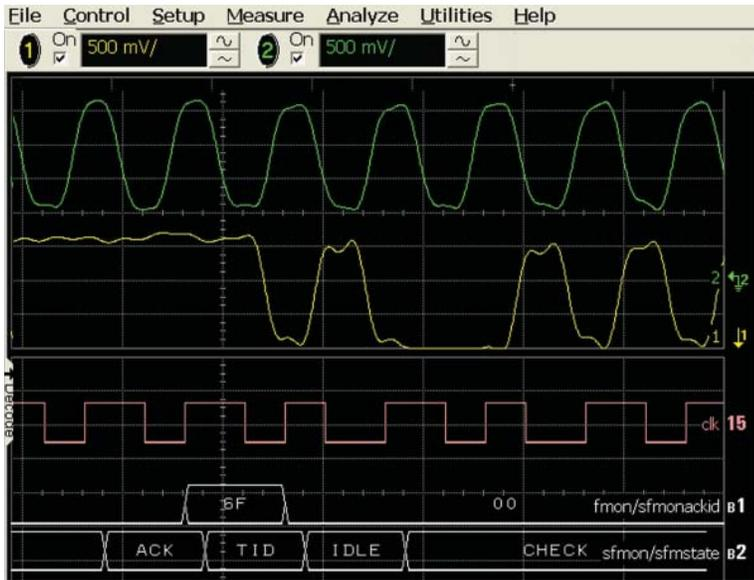
Use the timing channels to evaluate control signal relationships and data buses up to 16 bits wide. Use symbols to more quickly interpret waveforms.
