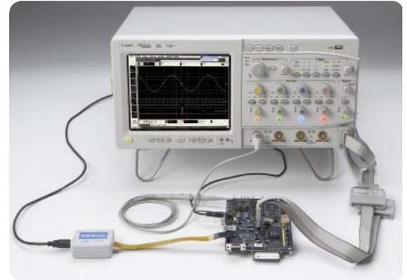
Designing with Altera or Xilinx FPGAs? Use the FPGA dynamic probe for rapid internal FPGA measurements. Using I<sup>2</sup>C, SPI, or CAN? Use the digital channels to acquire and decode these buses, preserving analog channels for other time-correlated measurements.
