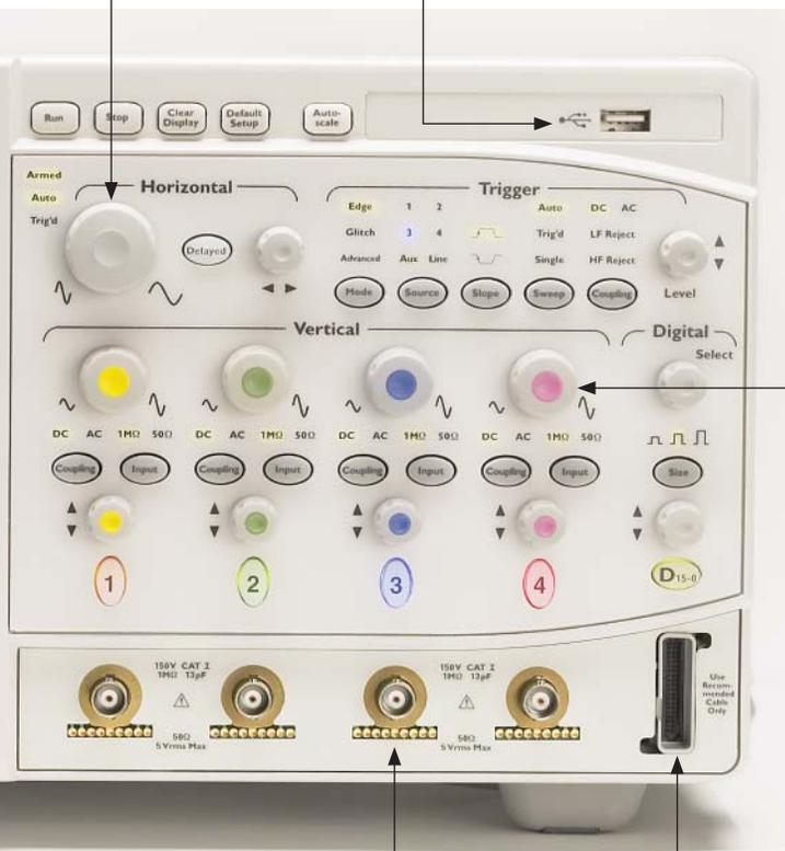
● **AutoProbe interface** completely configures your oscilloscope and provides power to various current and active probes, including InfiniMax active probes.
