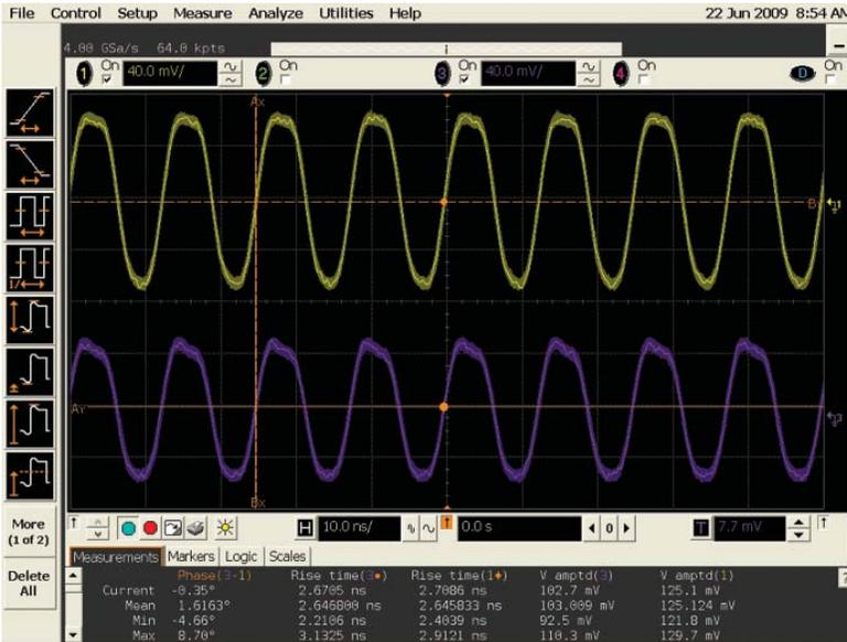
Up to 1 GHz bandwidth and 4 GSa/s high sample rates guarantee you'll see a good representation of the analog characteristics of signals you're testing.
