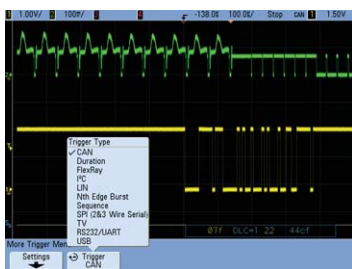
Trigger on and decode CAN serial packets.
