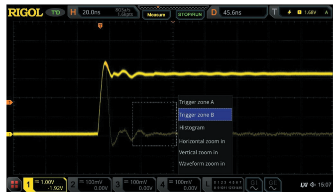
Draw a rectangle on the transient exception signal and select Trigger zone B.
