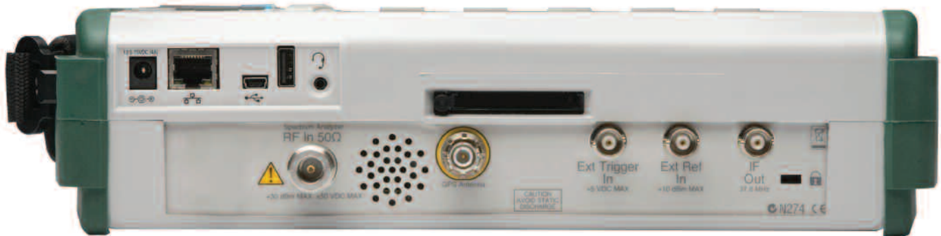
MS2723B and MS2724B Connector Panel
