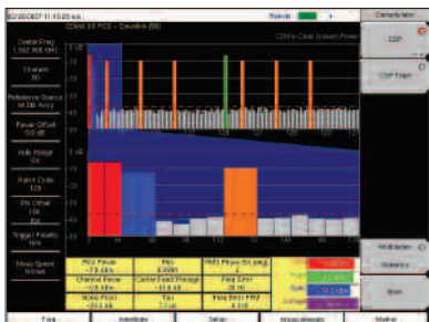
CDMA Code Domain Power measurement display
