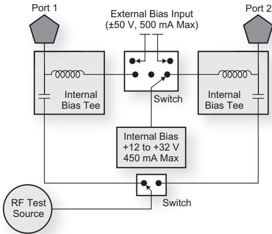
The VNA Master offers optional integrated bias tee for supplying DC plus RF to the DUT as shown in this simplified block diagram. Connectivity is also provided for external supply (instead of internal) to preserve battery consumption.
