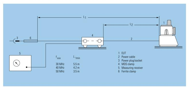
Test setup for measuring the disturbance power
