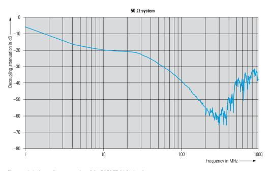
Characteristic decoupling attenuation of the R&S® EZ-24 ferrite clamp
