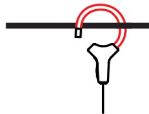
Close the coil. In order to optimize measurement quality, it is best to centre the conductor in the coil and to make the shape of the coil as nearly circular as possible.
