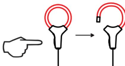
Open it, then place it round the conductor through which the current to be measured flows (only one conductor in the sensor).
