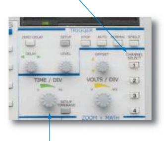
Adjust the **Time/Div** and SMARTMemory automatically assures the maximum resolution for each timebase setting.
