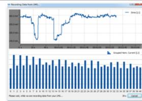
The tests performed by LMG Test Suite are in accordance with the currently valid edition of EN 61000-3-2/-12, EN 61000-3/-11, IEC 62301 and EN 50564. Measurements according to ECE R-10.4 Annex 11 (electromagnetic compatibility of vehicles), for example, are also possible.
