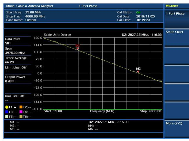
Cable and antenna test — 1-Port Phase
