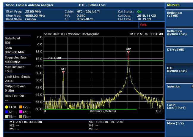
Cable and antenna test — Distance to Fault
