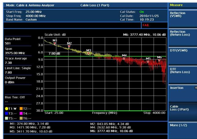
Cable and antenna test — Cable Loss
