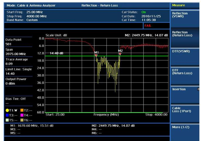
Cable and antenna test — Reflection
