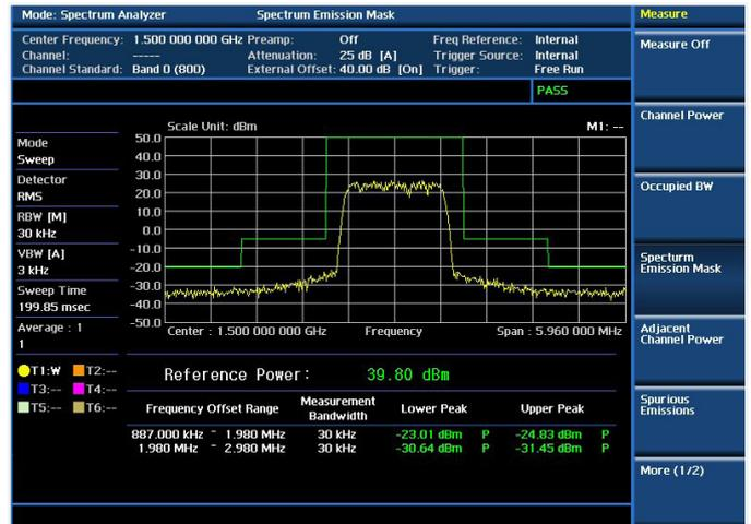
RF test — Spectrum Emission Mask
