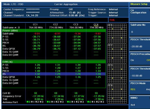
Modulation analysis — Carrier Aggregation
