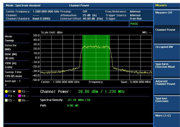
**Occupied BW** measures the frequency bandwidth that contains the specified percentage of the power, the total integrated power, and the occupied power with pass/fail results for the defined bandwidth.
